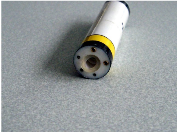
Figure 10.4: Bottom View Showing Silicon Rubber Sealing
